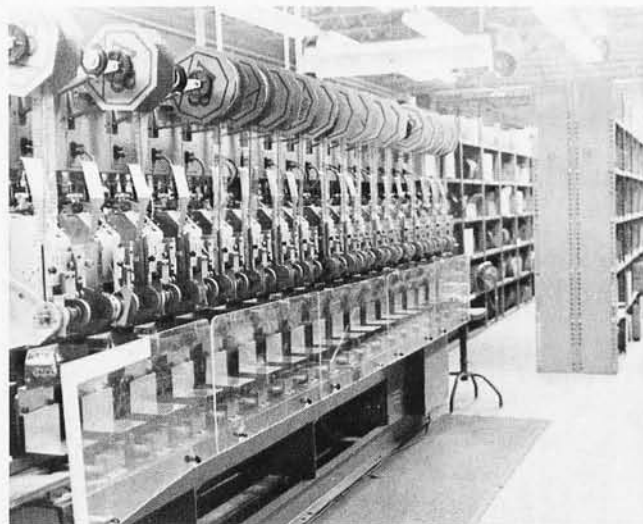
Photo 5: One point which many might overlook, but technology freaks can't ignore, is the specialized equipment which gets built when a firm has a large manufacturing operation. Here is a prime example of several very interesting cases of manufacturing automation at Heath: a machine which collates resistors prior to packing. Each reel holds a supply of resistors mounted on tape strips which many readers may have seen occasionally in surplus houses. The reel feeds a mechanism which removes the resistors from the tape on command and drops the resistor into a bin on a conveyor belt moving horizontally in a loop around the machine. The net result is that the human bag packers (not seen in this photograph) simply dump the properly collated resistor assortment from a bin into a bag and seal it, and have no need to physically handle each resistor. Such automation is possible only due to the uniformity of the resistors, and even then a machine tender is required to monitor occasional exception conditions.
