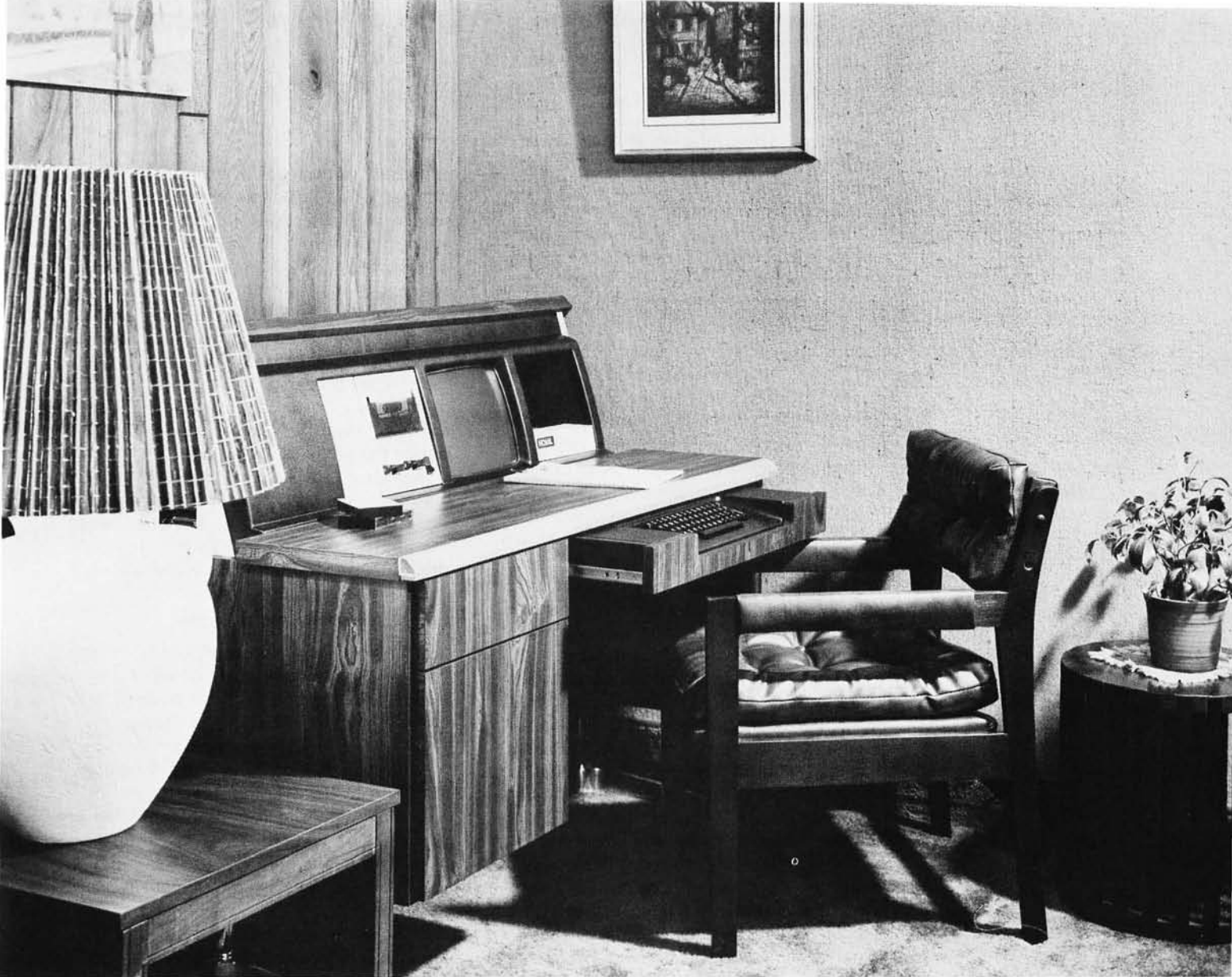
Photo 1: The Noval 760 is shown in this picture as it appears in its natural setting for use: unfolded in a living room, office or den. The console with display and cassette drive folds into the desk and the drawer with its keyboard closes, so that when not in use the Noval 760 blends into the decor as a desk-like woodtone piece of furniture.
