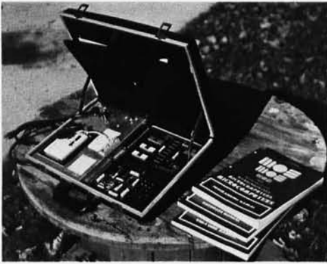
Photo 1: The author's new dress for KIM is shown in this shot taken with the briefcase opened. The unused area of the power supply cover is used to advantage as a place to mount prototyping boards for use in IO contexts with KIM.
